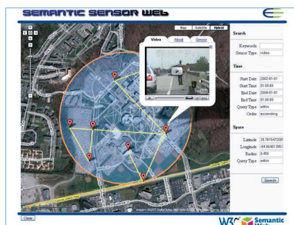
Figure 3. A semantic mashup with ability to show videos that capture events from police cruiser cameras with user queries on spatial region and time interval.
